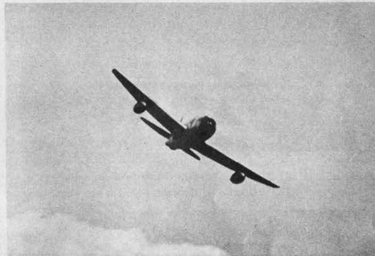
Okinawa-based P-47's may also be encountered over the Jap homeland. Long-range N model has greater wing span, squared-off wingtips.
